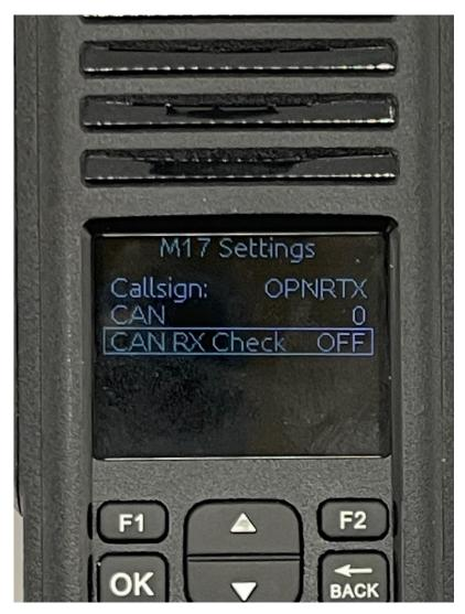
Use the up and down keys to select the value. The possible values are ON and OFF. When finished, press the OK key to lock it in. If set to OFF, then it acts like a promiscuous mode and will hear the other radio no matter what the CAN is set to. Using the Back key, you get to the following screen:
