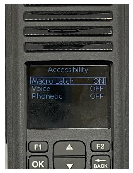
Use the up and down keys to select the value. The possible values are ON and OFF. When on, the macro menu latches after a 700ms press of the macro button (TK1). This allows the user to keep the macro menu active even when the side key is released, useful for the people having reduced mobility. When OFF, the user has to press the macro button at the same time as pressing the keys used in the macro menu.
