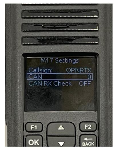
Use the up and down keys to select the value. The possible values are between 0 and 15. When finished, press the OK key to lock it in. The CAN is an abbreviation for Channel Access Number and is like a CTCSS number. If someone is transmitting to you and your CAN numbers do not match, then you will not hear them unless the CAN Rx Check is OFF. Pressing the OK key with the CAN Rx Check highlighted gets the following Screen:
