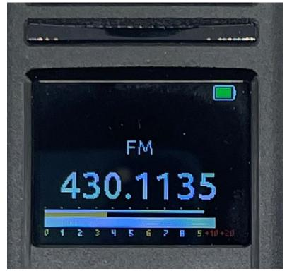
The frequency shown above is the receive frequency. When you press the PTT, the receive frequency is replaced by the transmit frequency.
