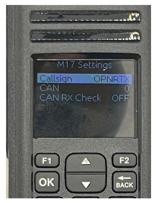
Us the up or down arrow to select the parameter you want to modify and then press the OK key to start the modification process.
