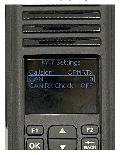
Pressing the OK key with the CAN Rx Check highlighted gets the following Screen:
