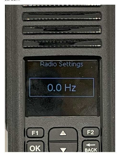
Use the numeric keys to enter your desired offset. Press the OK key to lock in your value.
