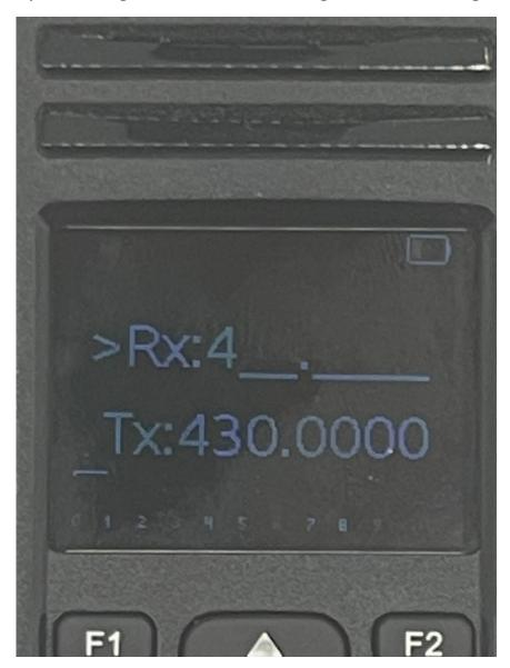
This screen requires you to put in a total of 7 digits for both the Rx and Tx frequencies. After you put in the 7 digits for the Rx frequencies, a copy of the Rx frequency will be copied to the Tx frequency as shown below.
