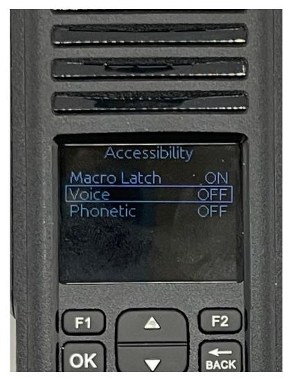
Use the up and down keys to select the value. The possible values are ON and OFF. This control the various levels of voice prompts for vision impaired operators. By default, voice prompts are off. The other steps are: keyboard beeps and then three different levels of spoken prompts with increasing verbosity.
