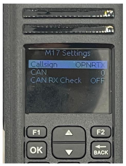
Us the up or down arrow to select the parameter you want to modify and then press the OK key to start the modification process. Pressing the OK key with the Callsign highlighted gets the following Screen:
