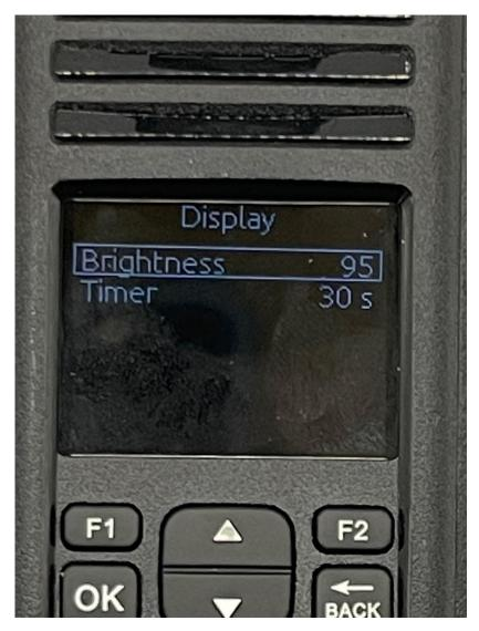
Use the up and down key to select the value you want. The values you can select is between 5 and 100 in increments of 5. The higher the number the brighter the display.
