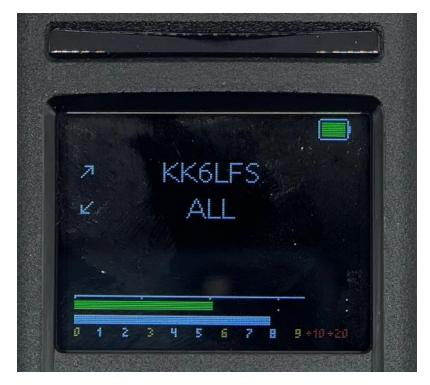
The battery on the top right of the screen shows the charge of the battery. If it is all green, then the battery is fully charged.
