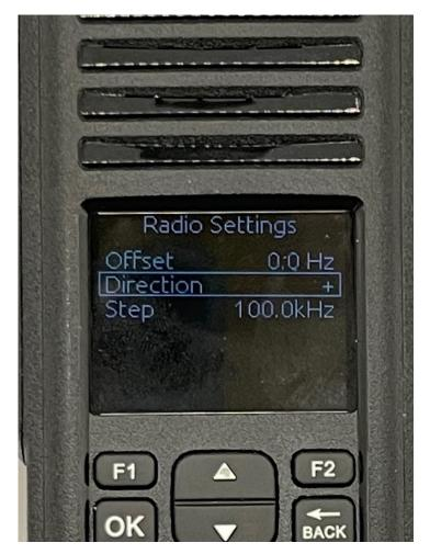
Use the up and down arrow to select either "+" or "-". Use the OK key to lock in the value.
