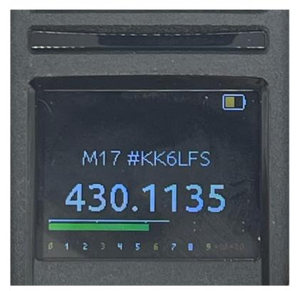
The battery on the top right of the screen shows the charge of the battery. If it is all green, then the battery is fully charged.
