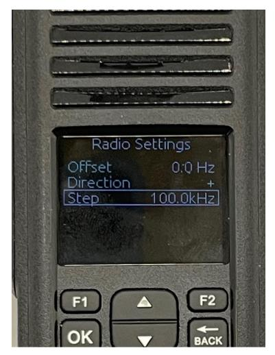
Use the up and down arrow keys to select the step value. Use the OK key to lock in the value. The possible values are:
