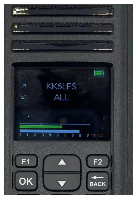
The destination address can be any address between 1 and 9 characters. The possible characters that can be entered are defined below:
