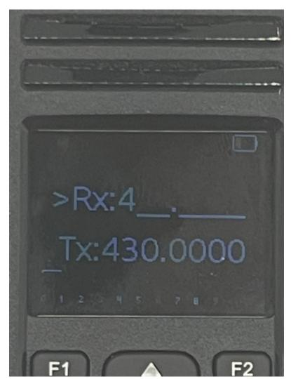
If you press the OK key before putting in all the digits, the radio will pad the rest of the digits with zeros. As an example, if you put in 4 like the screen above and press the OK key, the radio will give you a frequency of 400.0000. This screen requires you to put in a total of 7 digits for both the Rx and Tx frequencies. After you put in the 7 digits for the Rx frequencies, a copy of the Rx frequency will be copied to the Tx frequency as shown below.
