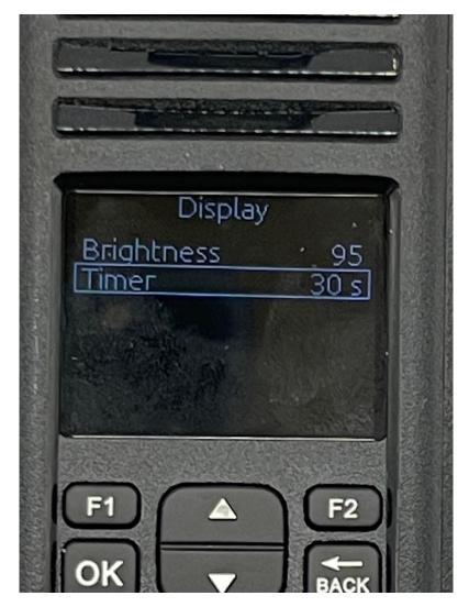
Use the up and down key to select the value you want. The possible values are shown below. Setting to off keeps the display always on.
