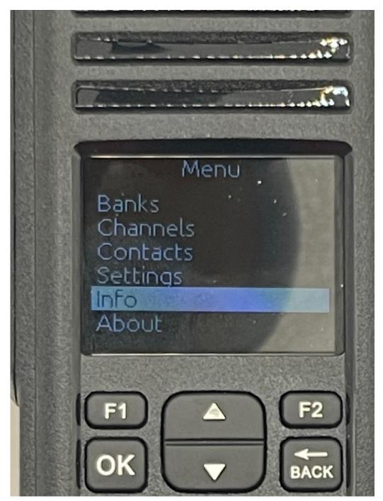
Use the up and down keys to select the feature you want. In a later firmware version, GPS was added. Then either the top of botton entry is not shown dependent on the scroll position.
