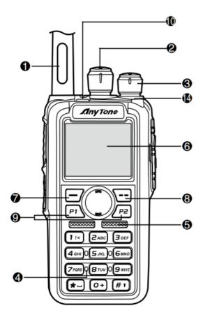
Press 7 (Menu) key to enter the menu, press key to the Device Info and enter into the menu to check the hardware version.
