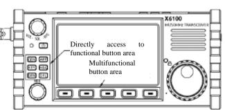
3. After selecting a function, rotate the large knob to adjust the corresponding parameter values. Adjustment parameters are displayed in the red character section in the function menu tag.
