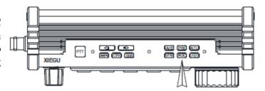
1. Press [AGC] key at the bottom of the screen in a short time, enable/ disable or select different AGC modes and circulate them in the following order:
