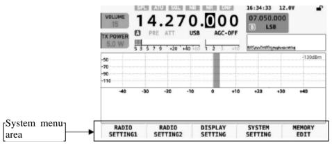
The system menu area is located at the bottom of the screen and is used to set or adjust some general parameters.
