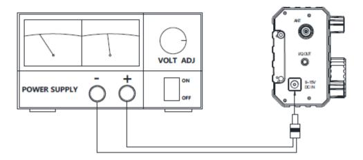
■ EMC magnet ring can be applied on power lines to prevent external disturbance from entering radio via power lines and radio-frequency interference in radio from radiating externally via power lines when external power supply is adopted for X6100. Magnet ring shall be installed at the side closing to radio to greatest extent.
