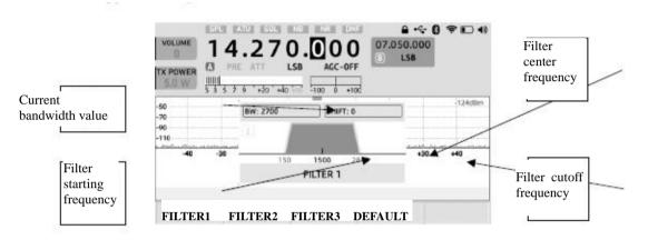
Filter Adjustment Schematic Diagram
