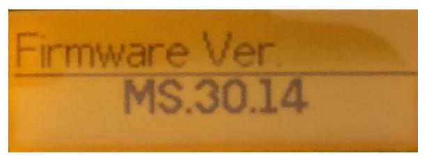
The firmware version for this CS800D radio is MS.30.14. At the time this application note was written, the latest firmware was version MS.30.16.
