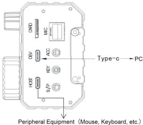
1. As shown in the figure above, connect the Type-C cable to the DEV port on the right side of the X6100.
