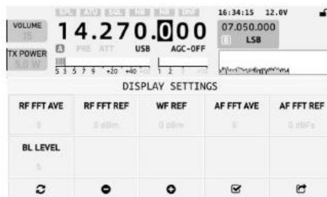
RF FFT AVE: settings of displayed average of radio frequency spectrum
