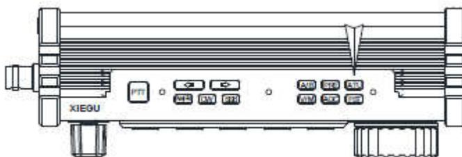
1. Short press [ATU] button to connect with built-in antenna tuner. There will be an antenna icon at the top of screen.
