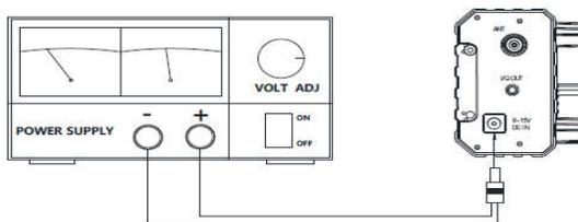
■ EMC magnet ring can be applied on power lines to prevent external disturbance from entering radio via power lines and radio-frequency interference in radio from radiating externally via power lines when external power supply is adopted for X6100. Magnet ring shall be installed at the side closing to radio to greatest extent.
