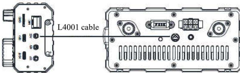
After the X6100 connects with XPA125B power amplifier and antenna tuner AIO through the L4001 cables, the output power can be expanded to 100W.
