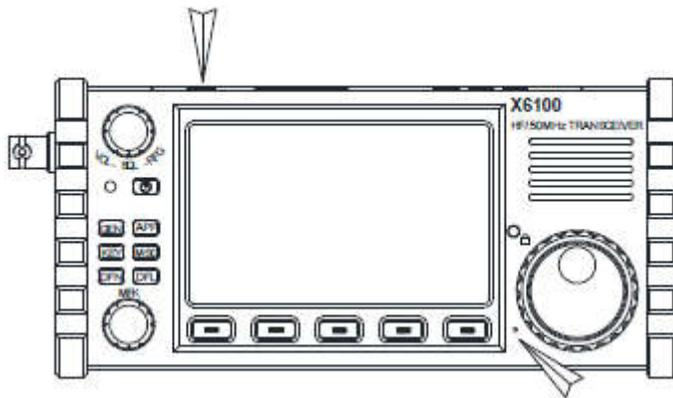
1. Press the PTT button on the top of the device and speak to the built-in microphone hole at the left of large knob to transmit voice.
